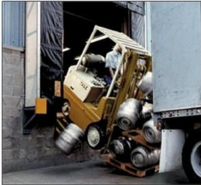
**4. Secure dock plates.** Unsecured dock plates can move over time. This can result in sudden stops or load disruption if the forklift wheels get stuck between the dock and the truck bed. Portable dock boards should be secured to prevent them from moving. For example, some dock boards have pins that are inserted into the sides to prevent the board from shifting toward the dock or trailer. Portable dock boards should also have handles for safe placement and removal.
